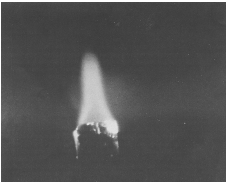
Fig. 2. Glycine emerging from the electrophoresis capillary into the reagent reservoir of the free-solution reactor, fiber optics illuminating fluorophore from side ( 1 \cdot 10^{-3} M glycine continuous injection 30 kV).
